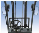
C-JJ wide view mast for clear front operator visibility
