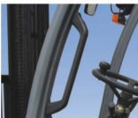
Large operator hand assisted access grip
