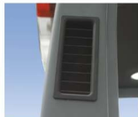
Top air inlet through canopy for cleaner air to engine
