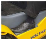
Wider operator foot rest for safer entry & exit
