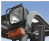
Protective light guards prevents damage
