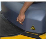
Lever for smooth opening of engine hood
